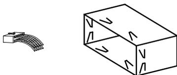
Slide the radios installation sleeve into the mounting kit. (some sleeves may be marked with "TOP" to note the top of the sleeve)
