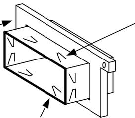
When the installation sleeve is fully inserted and the front edge or lip is seated against the front face of the installation kit, bend the tabs of the installation sleeve behind the rear surface of the installation kit to secure the installation sleeve. Bending the tabs secures the sleeve to the kit.
